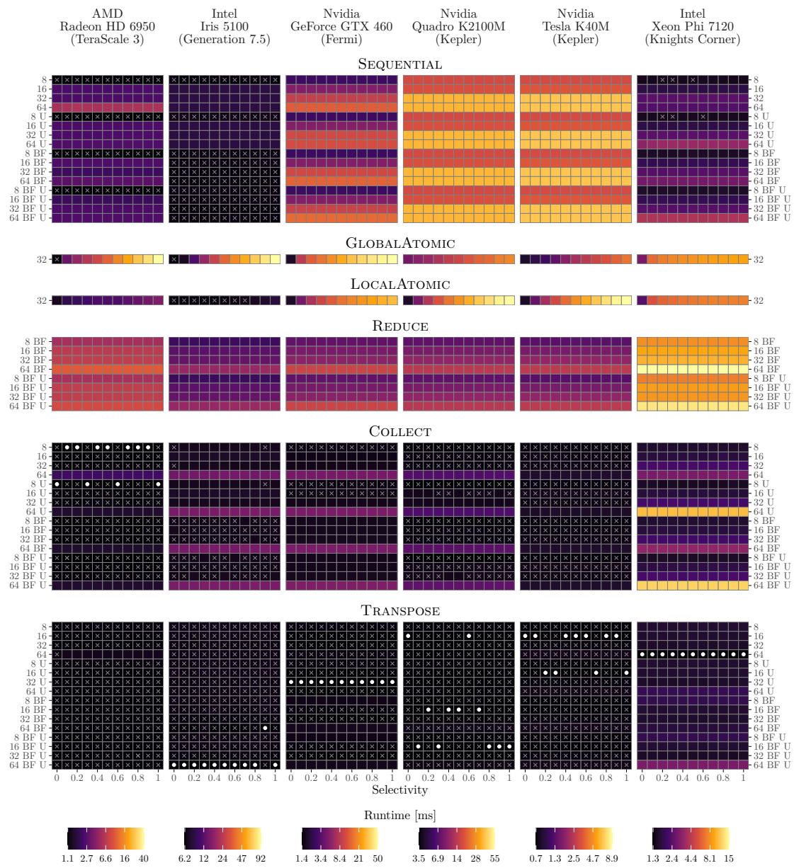
Figure 3.2.: Selection operator performance on different processors (continued from previous page, GPUs and Intel Xeon Phi).
